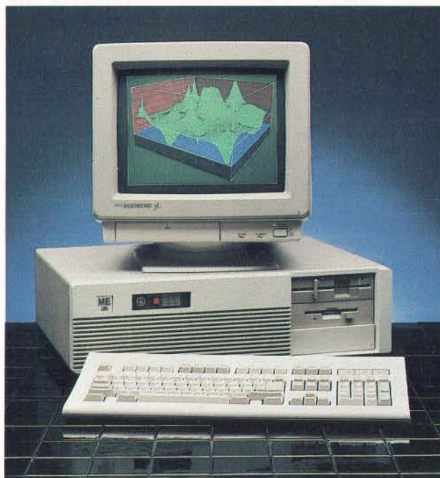
The 33-MHz Micro Express ME 80386 with optional floppy disk drive and VGA monitor.
